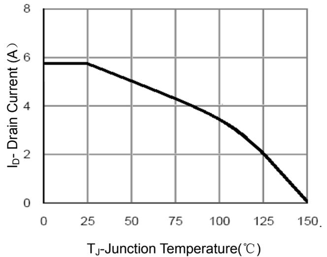
Figure 4 Drain Current
