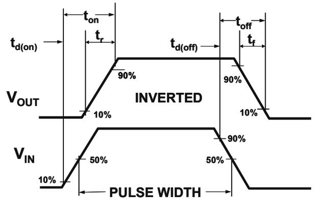
Figure 2: Switching Waveforms
