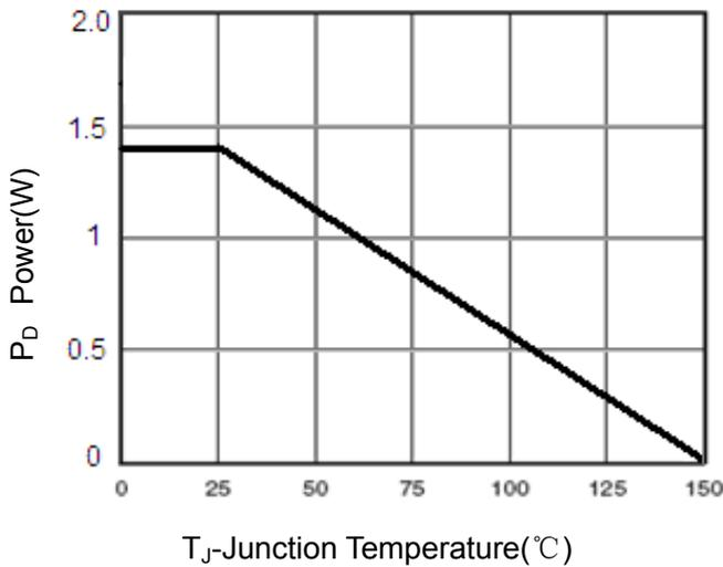
Figure 3 Power Dissipation
