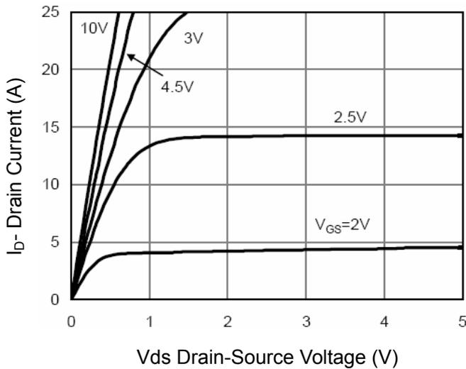
Figure 5 Output Characteristics
