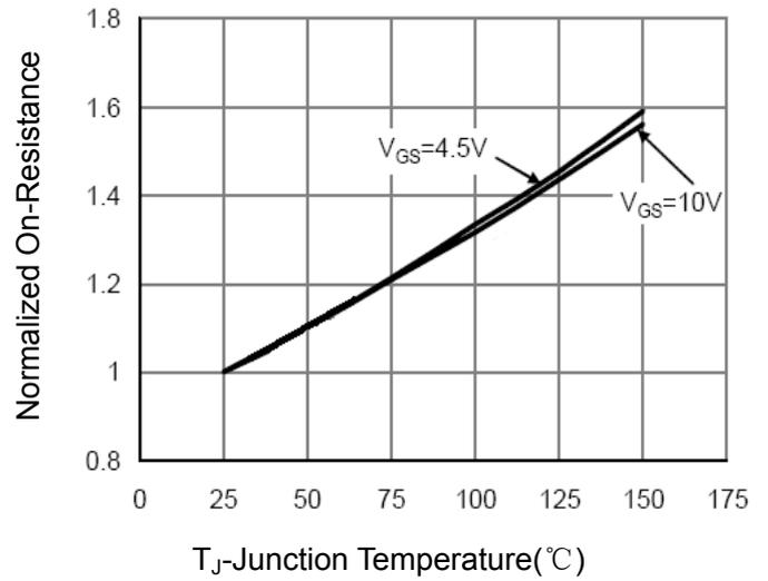
Figure 8 Drain-Source On-Resistance
