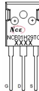
Marking and pin assignment
