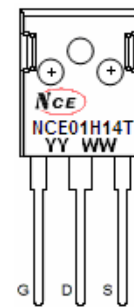
Marking and pin assignment
